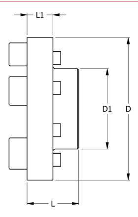
D = 400 D1 = 200 L = 160 L1 = 56 Max bore = 120 Torque (N m) = 10300
